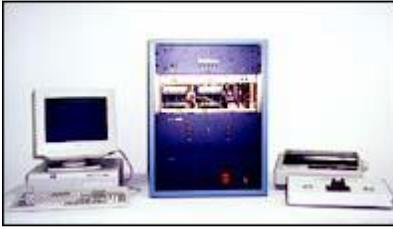
The CV400 tests silicon Transient Voltage Suppressor (TVS) diodes, both uni-polar and bipolar. The waveform used for the main test is the 10/1000 $\mu$ s waveform.
