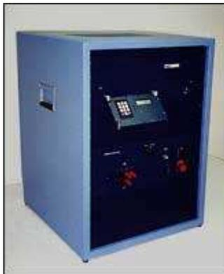
The PLS500 automatic tester is designed primarily to do SURGE testing either as single pulses or with Forward and Reverse bias, according to methods 4066-1 or 4066-2. In addition, it can also test VF with rectangular pulses and THERMAL RESPONSE either in DVF (mV) or degrees per watt. All three test types may be performed in a single test program.
